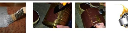
Applied by immersion, brush, swab for protecting metal sheets, metal and bearings etc.
